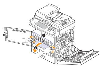
6 Pull the used imaging unit out of the machine using the handle on its bottom.
